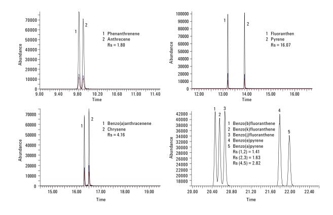
Figure 2. Resolution of Critical isomer Pairs with the DB-EUPAH column, 20 m × 0.18 mm × 0.14 µm (Agilent p/n 121-9627).
